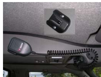
Install microphone clip on acute angle
